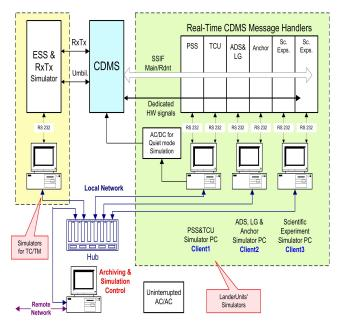
Figure 3. The structure of LSS network
